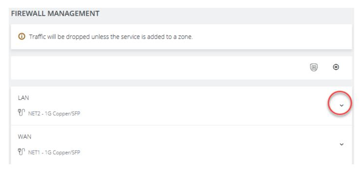
To add a source address filter for a zone, select the **edit zone** option under the required zone, which opens the **edit zone page** where source address filters can be configured.
