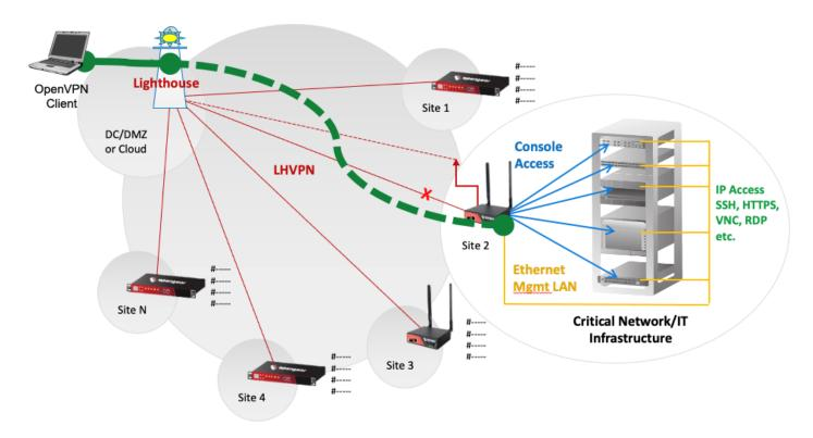
In the diagram, the client PC has a virtual tunnel interface with a route to the yellow management network, and the user can access any target IP devices on the yellow network using their real IP addresses.
